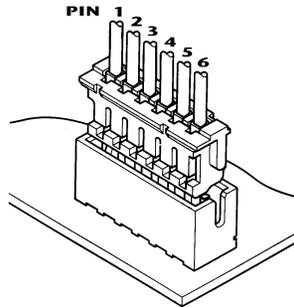
Compatible speed control must use the six position JST header part number X-6B-ZR-SMX-TK (where the X denotes the style of the header), or equivalent.
